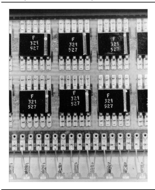
Micrologic chips installed on "Logic Stick"
