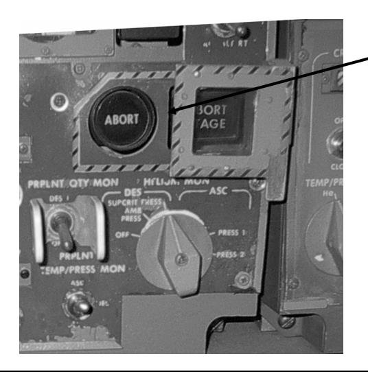
Pressing the Abort button automatically switches software to Abort program
