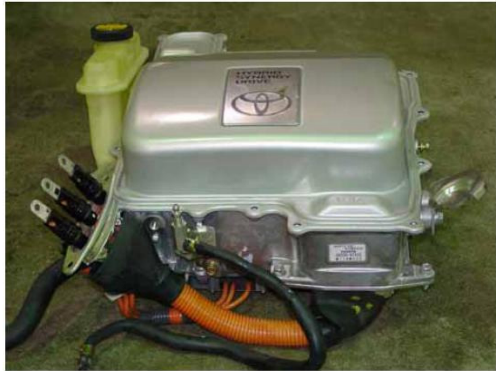
Fig. 2.9. 2004 Prius inverter and converter unit.
