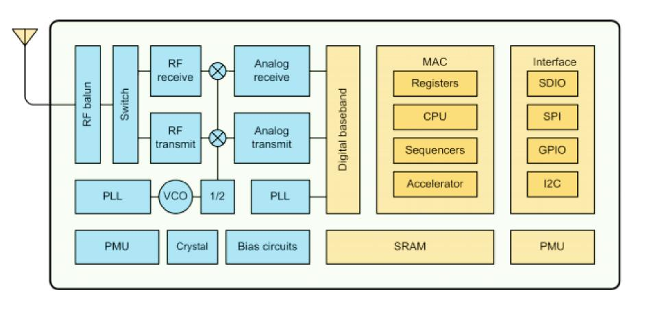
Figure 1 ESP8266EX Block Diagram
